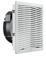
GF series exhaust filter and filter fans represents a side-mounted cooling solution with filtered ambient air to maintain optimum ventilation inside the electrical cabinets. Characterized by a mounting system with jacks for thick wall application (up to 8mm extensible up to 16mm by cutting the jacks) in both plate and plastic enclosures, and a hinged opening for a filter media replacement in seconds.
